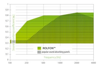
ROLFON™ absorbs noise 2 octaves broader than any other absorbing material (including baffles or mineral wool ceiling boards).
