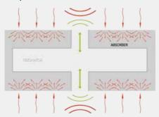
The construction guarantees the best impact resistance and allows for easy arrangement of ROLFON<sup>™</sup> rolls into groups of any shapes and configurations. The roll, including latches, weights less than 1.5kg (3.3lb).
