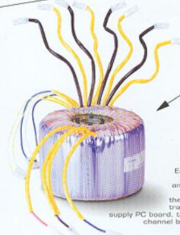
Each module has been designed for fast and easy servicing [just in case you need it ...]: the enormous toroidal power supply PC board, the two power channel bars...
