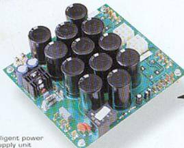
The intelligent power supply unit contains a total capacity of 600.000  $\mu$ F for the HC 2000 and 120.000  $\mu$ F for the 3.200 model: an incredible energy store for your music!
