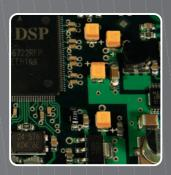
The integrated digital processor is based on a state of the art 32 bit, floating point DSP running at 96 KHz sampling rate. The calculation capacity largely exceed the processing needs and the DSP is never pushed to the limit. Crossover and equalization of the transducers, limiter, system presets: high pass, air absorption and cluster size corrections.
