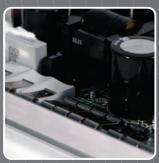
The TTL33-A is powered by a 750 watt switching power supply and 3 digital amplifiers: 500 watt mid-bass, 500 watt midrange and 250 watt compression driver. 750 watt power for the TTL31-A: 500 watt low frequency and 250 watt high frequency. The result is very high output, extremely low distortion and natural sound.
