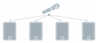
If you need several loudspeakers you can drive as many move 100 as you like from only one transmitter, within the possible range of the transmitter, heavily dependent on the environment.
