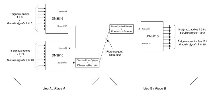
Exemple n°2: transportation of 8 audio signals from 1 place to 4 distant places through optic fiber link
