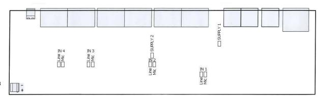
There are two possible configurations for inputs IN 1 to IN 4: Line input (0 dBm) or Micro input (-52 dBm). In addition, when audio inputs 1 and 2 are set to Micro, these can be supplied a phantom power supply for powering electret microphones. Whichever configuration is to be used, follow the procedure below to set the inputs according to the desired application.
