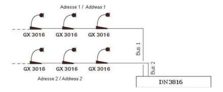
The GX 3016 consoles connected to bus 1 must be set to address 1 and the consoles connected to bus 2 to address 2 (see figure above). To set the addresses on the GX 3016 consoles, refer to the GX 3016 User Manual. Use the RJ45 cable to connect up the GX 3016 consoles (refer to the wiring details below).
