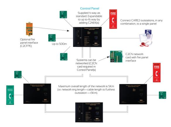
Up to 16 panels can be placed on the network (2 of these can be control panels, one of which will act as a slave unless activated as the master during an emergency).
