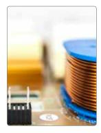
The system includes a high-level crossover network that features markedly lower (than conventional) induction values in series with the woofer. The benefits are reduction in delay, reduced phase shift and superior transient response. The high power internal passive filter provides crossover protection and equalisation. The system is able of producing a Max SPL of 137 dB and handles 900 Watts AES (LF) + 110 Watt AES (HF).
